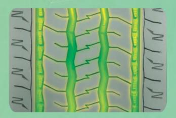
SSHT Shoulder Stiffness Hold Technology (SSHT) - Less uneven wear
